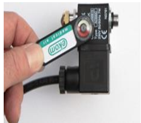
Fig. 22: Check of solenoid valve operation
