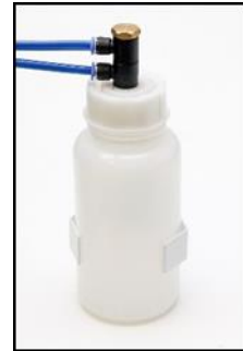
Fig. 18: Check of condensate collection vessel
