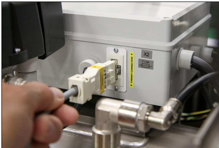
Fig. 13: Connect the cabinet to the compressor
