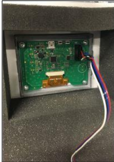
Fig. 17: Connecting the display connector
