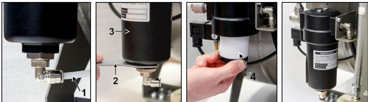
**Fig. 19: Filter element replacement**
