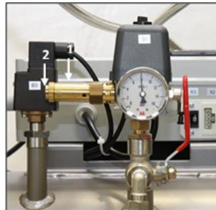
Fig. 17: Check of safety valve
