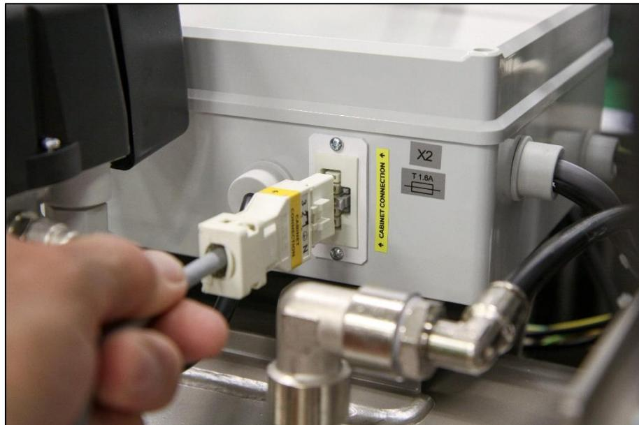
**Fig. 13: Connect the cabinet to the compressor**
