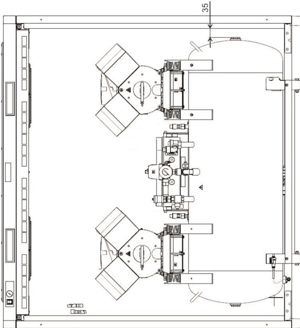
**Fig. 6: Placement of the compressor in the cabinet**
