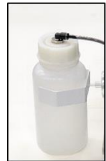
Fig. 16: Check of the condensate collection vessel
