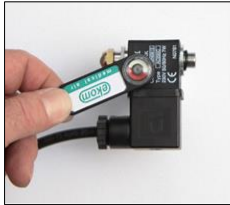
Fig. 19: Check of solenoid valve operation
