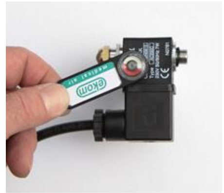
Fig. 28: Check of solenoid valve operation
