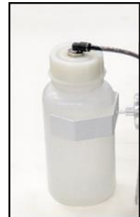
Fig. 15: Check of condensate collection vessel
