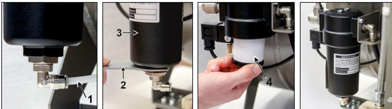
Fig. 18: Replacement of filter element
