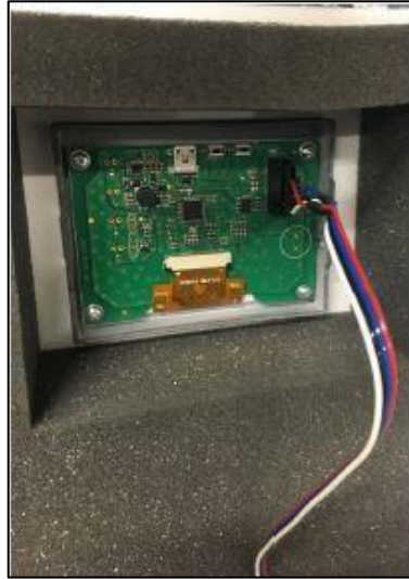
Fig. 17: Connecting the display connector
