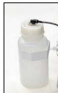
Fig. 17: Check of condensate collection vessel
