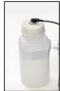
Fig. 16: Check of the condensate collection vessel
