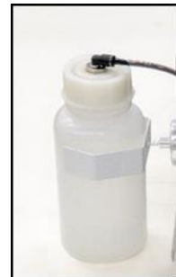
Fig. 5: Check of condensate collection vessel
