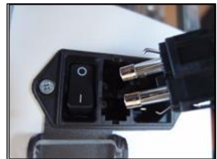
Fig. 25: Replacement of fuses
